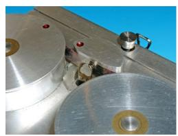
Close-up view of the keyer contact and top deck latch.
